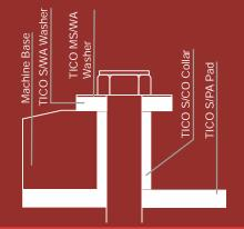
Floor mounted plant- bolt secured Location of TICO S/PA pad utilising floor bolts together with TICO S/CO collars and TICO S/WA and MS/ WA washers.
